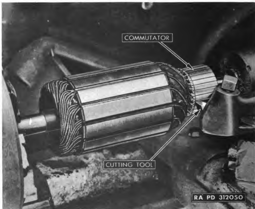
Figure 23—Turning Commutator in Lathe
